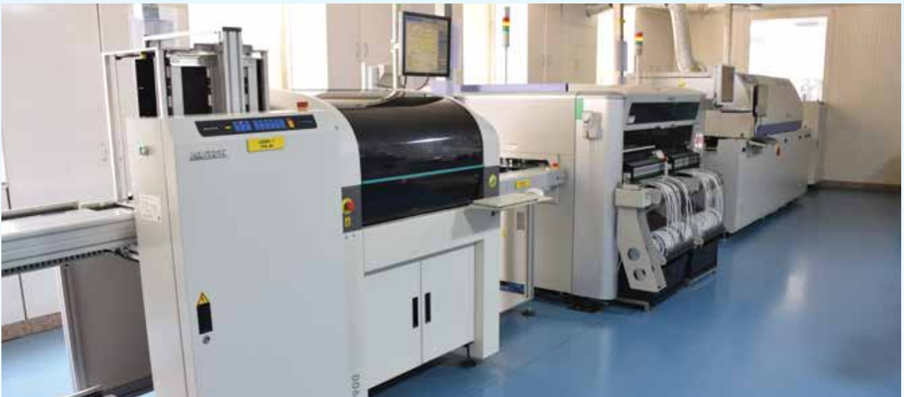
Jain Solar Controller and PCB Manufacturing plant, (SMT line fully automatic) Green Energy Park; Jain Valley, Jalgaon.
